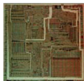
Intel 8086, 1978, 33mm 2 10Mhz, 29K transistors, 3u
