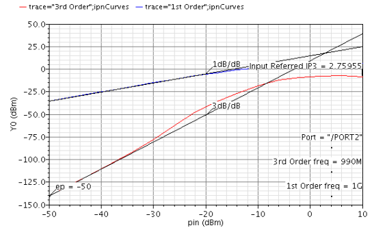
Fig. 7: IIP3 of the proposed balun-LNA before and after utilizing the proposed linearity improvement technique with 10 MHz spacing.
