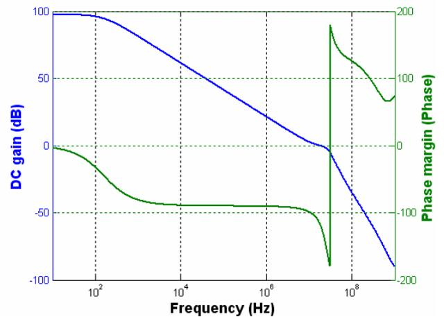
Fig. 4: Simulated open-loop frequency response of the amplifier.
