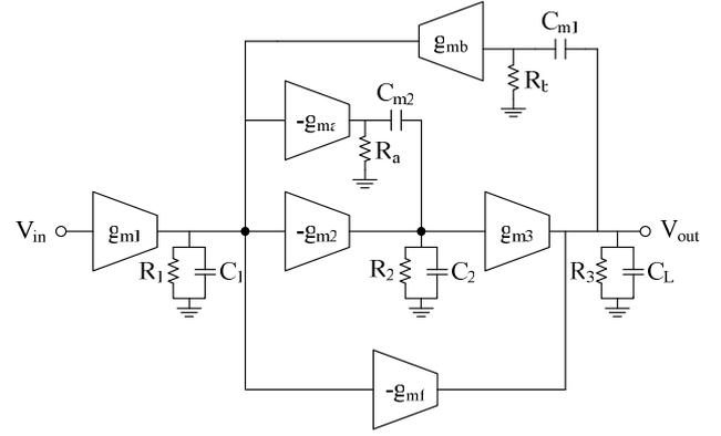
Fig. 1: Proposed dual-active capacitance compensation three-stage amplifier.
