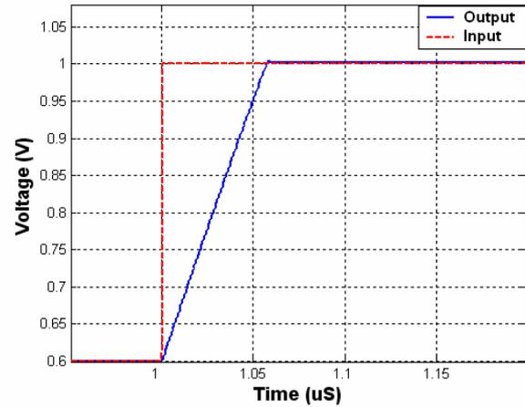
Fig. 5: Simulated transient response of the amplifier.
