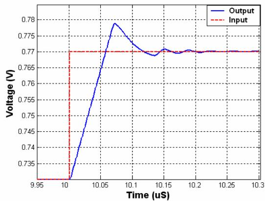
Fig. 6: Small-signal input-output characteristic of the amplifier.
