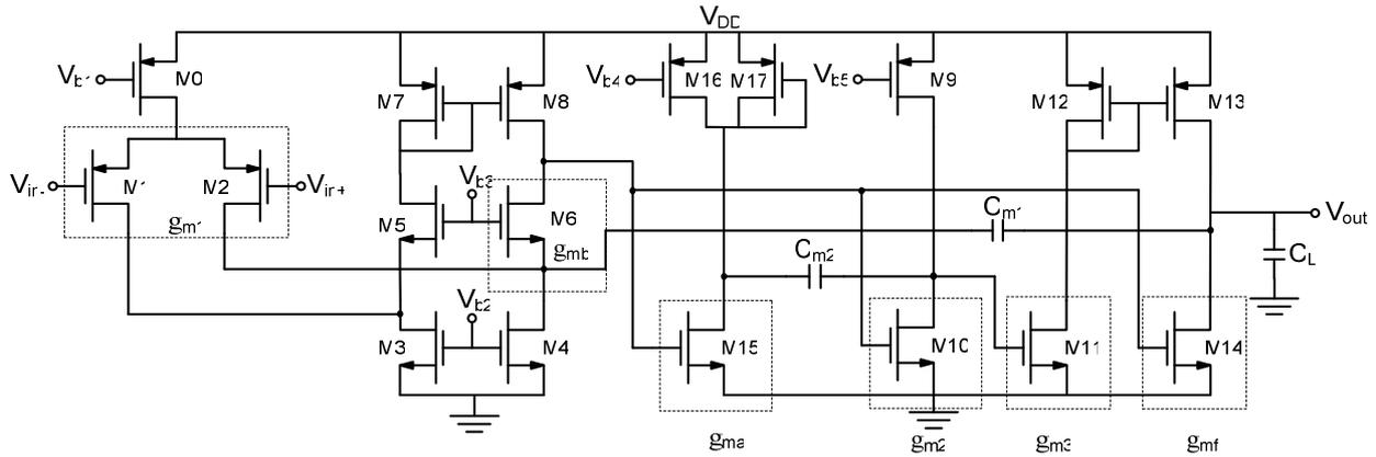
Fig.3: Circuit implementation of a three-stage.
