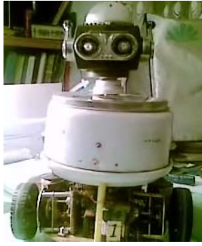
Fig.5 AI Graph search Algorithm for navigation of first Iranian pedagogic robot called PARS-1B. Developed by Author, in Sharif university of technology, E.E. Dept., year 1986 [1,18]. Both PARS-1B and Sophia robots are logic Boolean machines which can not think.
